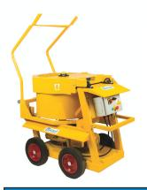
The Mixit 60 forced action pan mixer has been developed specifically for heavy duty industrial applications. The mixing pan is driven through a gearbox by either diesel, petrol/gasoline, or electric motor. As the mixing head is lowered, the machine automatically starts, and then stops when the head is raised. A steel grill panel allows bagged material to be introduced throughout the process. Once mixing is complete the mix can easily be emptied using the tipping device.
